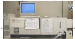
Aviv CD spectropolarimeter
