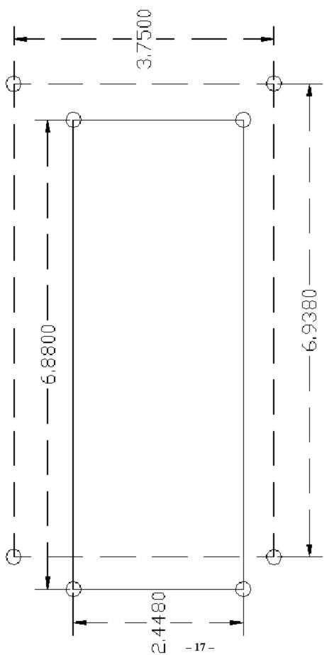
Base Mount (8314-7) = dashed lines Please Note - Template size may vary on different printers. Make sure your holes are marked per the dimensions on the template. Note: All dimensions in inches
