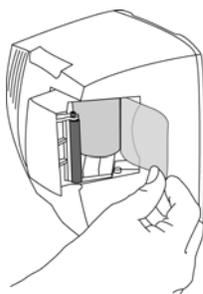
3. Place the roll of paper into the compartment so that the end of the paper comes off the right-side of the roll (paper is wound around the roll clockwise). Place the roll of paper in the holding bracket that is integrated in the door of the printer, making sure the paper extends out of the printer cavity at least two inches.
