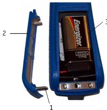
3. Disconnect and remove the battery (3).
