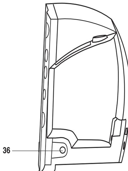
36. External DC power socket: used with GE-approved AC-DC power converter only. Refer to Appendix B, “[Accessories](#)” for the part number of the approved power supply.
