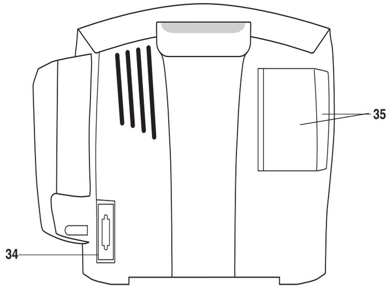
34. Host communications port (15 pin D-type RS-232 serial port) for use only with equipment conforming to IEC 60601-1 or configured to comply with IEC 60601-1-1. The Exergen scanner connects to this port.
