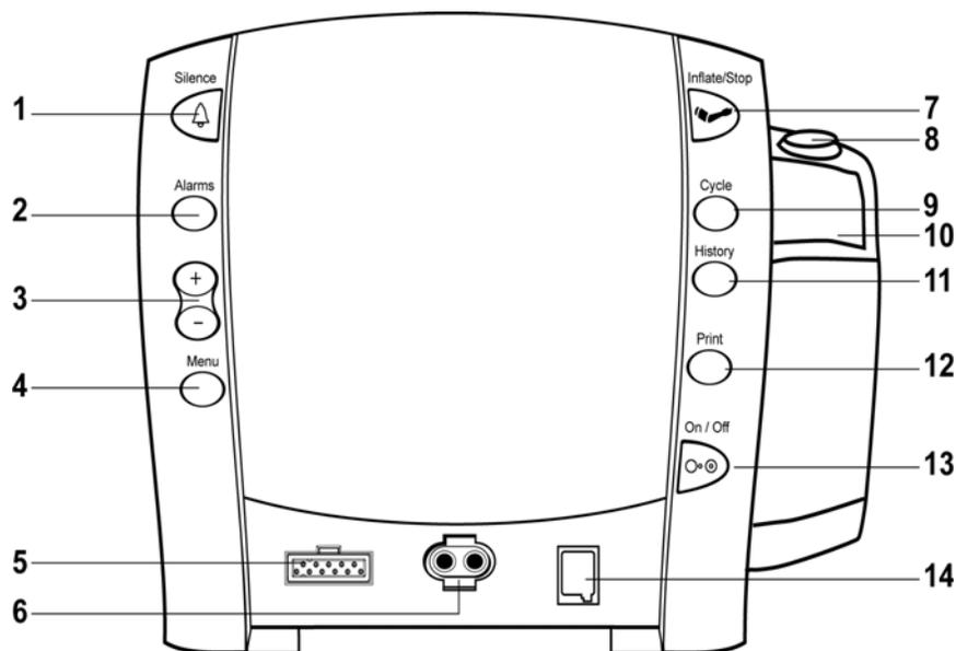
1. **Silence** button: mutes audible alarms. Any other active alarm that can be acknowledged is also cleared and the alarm condition is reset whenever this key is pressed. When pressed, the alarm silence indicator (bell) lights solid red to indicate that audible alarms have been silenced for 2 minutes. Alarm silence can be cancelled by pressing the **Silence** button again.
