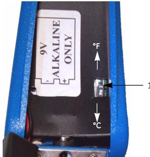
5. Replace the battery and cover, then tighten the screw.
