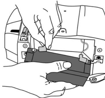
6. Then replace the cover, help card tray, and screws. Insert the external DC power converter plug into the external DC power socket and plug into an AC outlet.
