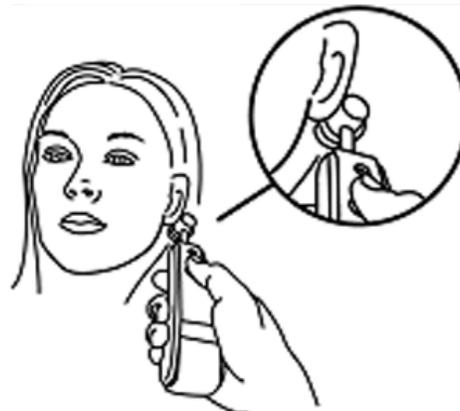
7. Release the red **On** button, read, and record temperature.
